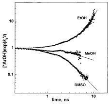
**FIGURE 12.** Time-resolved kinetics of **5SMN1** in alcohols and DMSO. "Corrected" experimental (dots) and theoretical (lines) \*ArOH decay.<sup>51</sup>
