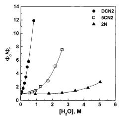
**FIGURE 10.** Stern—Volmer quenching of naphthol fluorescence by water in aqueous tetrahydrofuran.  $\Phi_f$  and  $\Phi_0$  are \*ArOH fluorescence quantum yields in solutions with and without water, accordingly.
