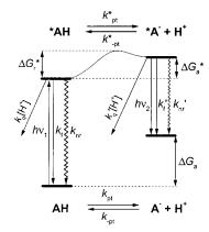
**FIGURE 1.** Proton transfer and decay processes in photoacids.
