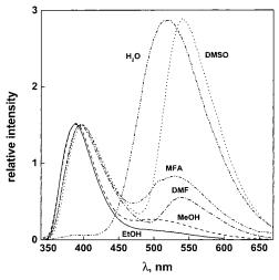
**FIGURE 7.** Fluorescence spectra of **5CN2** in solvents to which ESPT takes place: DMSO, dimethyl sulfoxide; MFA, *N*-methylformamide; DMF, *N*,*N*-dimethylformamide; MeOH, methanol; EtOH, ethanol.<sup>39</sup>
